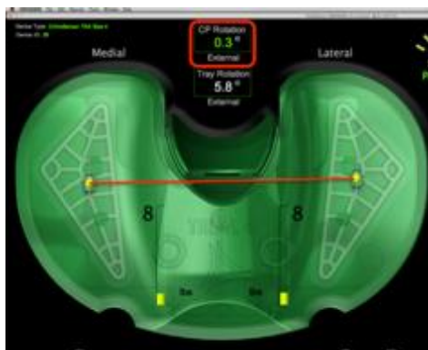
Figure 4. Sensor as displayed on graphical user interface. CP (Contact Point) Rotation degree [in red box] references the degree of tibiofemoral incongruity. Yellow circles correspond to femoral contact points. The number 8 represents total pounds of pressure in the medial and lateral compartments.
