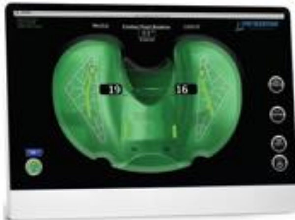
Figure 1b. Wireless graphical display of compartmental loads and tibiofemoral contact points in real time
