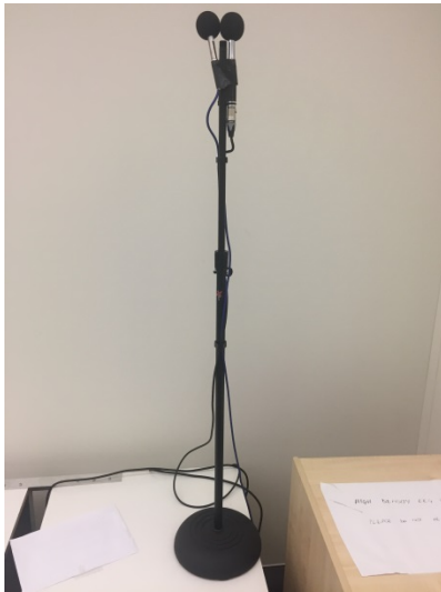
Figure 3. Microphone stand with infrasound and audible sound microphones
